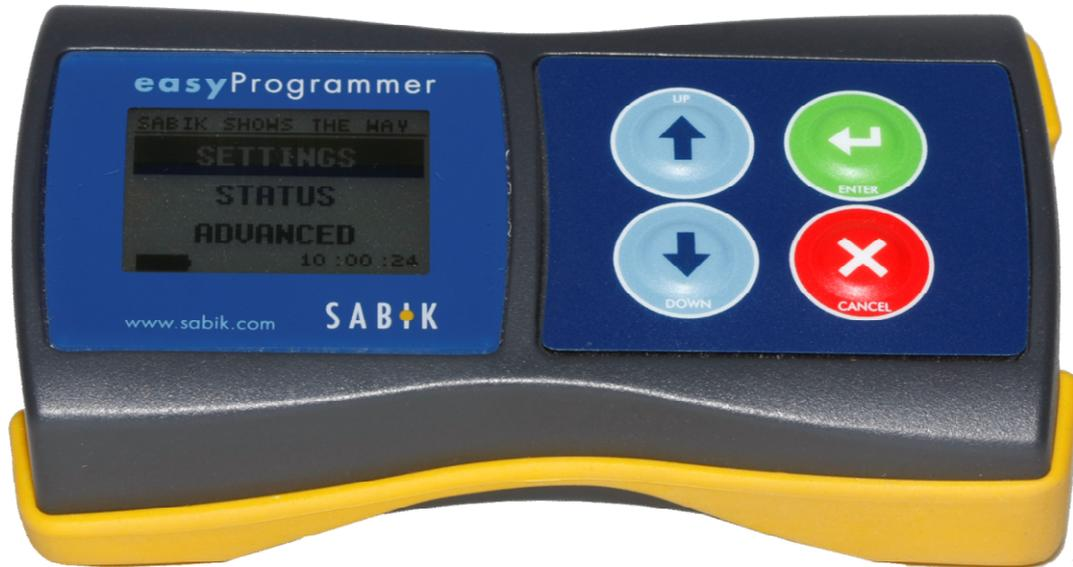
Sabik easyProgrammer is a stand-alone simple programmer for lanterns with an infrared-Interface. With the aid of easyProgrammer PC software, you can download/upload information to/from the handheld programmer to a Windows based personal computer. This is done using the SABIK Infrared USB interface (sold separately).
