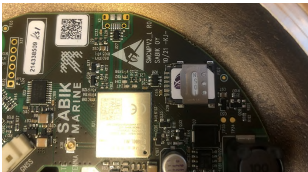
Figure 2 – Close the SIM card lock and slide it to the right in order to secure the SIM card
