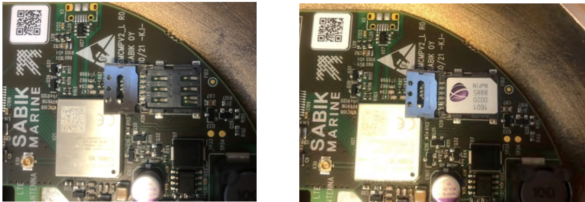
Figure 2 – Swipe left to unlock and lift up the SIM card holder and place SIM card in the holder
