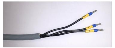
The VLB-44X is supplied with a 2 metre length of PUR 3-core 2.5mm<sup>2</sup> cable already sealed into the cable gland. If there is a need to shorten the power cable, ensure that the cable is resealed using heat shrink and marine sealant at the cut to prevent any moisture being able to enter the beacon.
