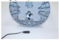
Step 2: Connect the Flash Technology-supplied charger accessory to the charge port.
