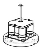
7. Lift out the battery pack. Remove the old black rubber gasket in the lantern base and replace it with the new one supplied.
