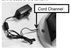
Step 4: Plug in the charger and let charge overnight. Wait a minimum of one hour and verify battery state-of-charge. The most accurate Battery Pack status reading is obtained when the lantern has been in a dark location and in "off" mode for at least 24 hours.
